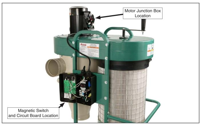
Figure 39. Electrical component locations.
